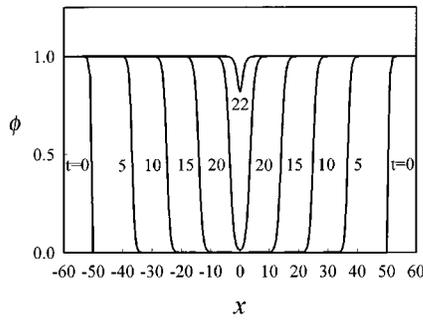
FIG. 1. Numerical simulation of Eq. (3) for  $m=2$ , exhibiting a pictorial representation of the exact solution (10). The two fronts propagate with velocity  $C=2$  in the opposite directions, and gradually disappear after collision.
